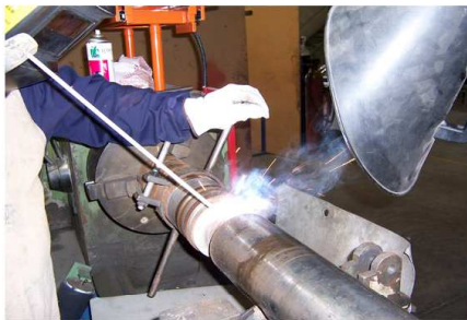
Bar of injection welding
