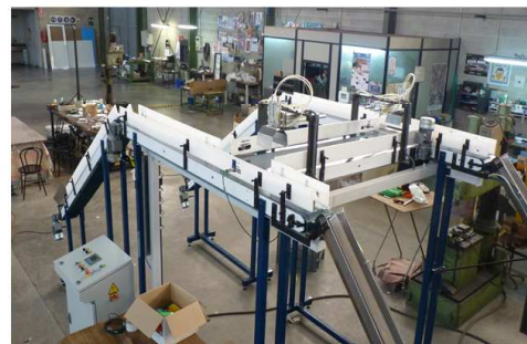
Elevated conveyor belts
